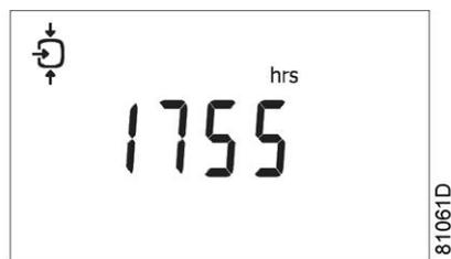
The screen shows the unit used <hrs> (or <x1000 hrs>) and the value <1755>: the compressor has been running loaded during 1755 hours.
