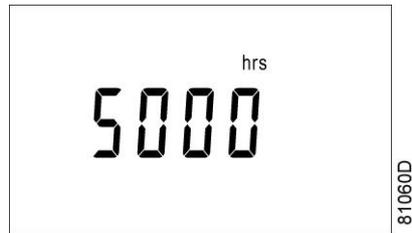
In the example shown, the screen shows the unit used (hrs) and the value (5000): the regulator module has been in service during 5000 hours.
