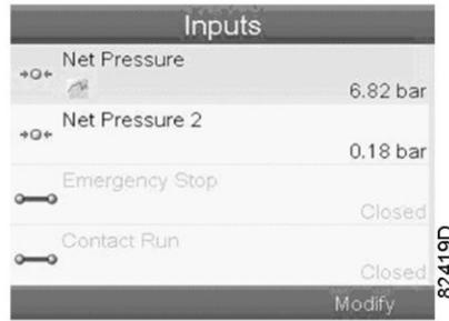
The first item in the list is highlighted. In this example, the Net Pressure is selected (chart icon). To change, press the Enter button again: a pop-up window opens:
