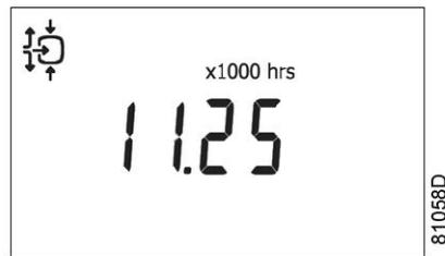
The screen shows the unit used (x1000 hrs) and the value (11.25): the running hours of the compressor are 11250 hours.
