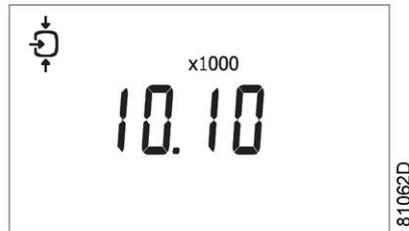
This screen shows the number of unload to load actions (x 1 or - if <x1000> lights up - x 1000). In the above example, the number of unload to load actions is 10100.
